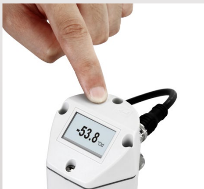
Alarm adjustment at dew point sensor
