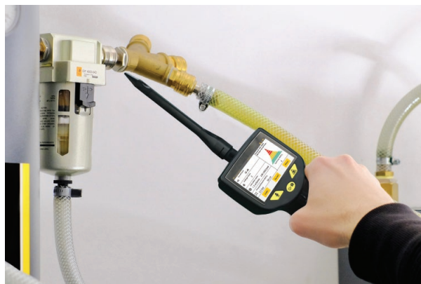
Leak detection with focus tube
